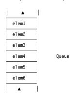
As the following figure shows, the data stack that REXX uses combines the techniques used in adding elements to stacks and queues. You can add elements on the top or the bottom of a data stack. Removal of elements from the data stack, however, occurs only from the top of the stack.
