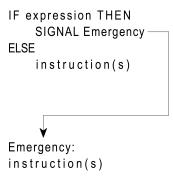
SIGNAL is useful for testing programs or to provide an emergency course of action. It should not be used as a convenient way to move from one place in a program to another. SIGNAL does not provide a way to return as does the CALL instruction described in the previous topic.
