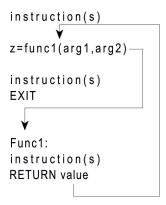
Both subroutines and functions can be internal (a label designates these) or external (a sublibrary member name that contains the subroutine or function designates these). The two preceding examples illustrate an internal subroutine named sub1 and an internal function named func1.
